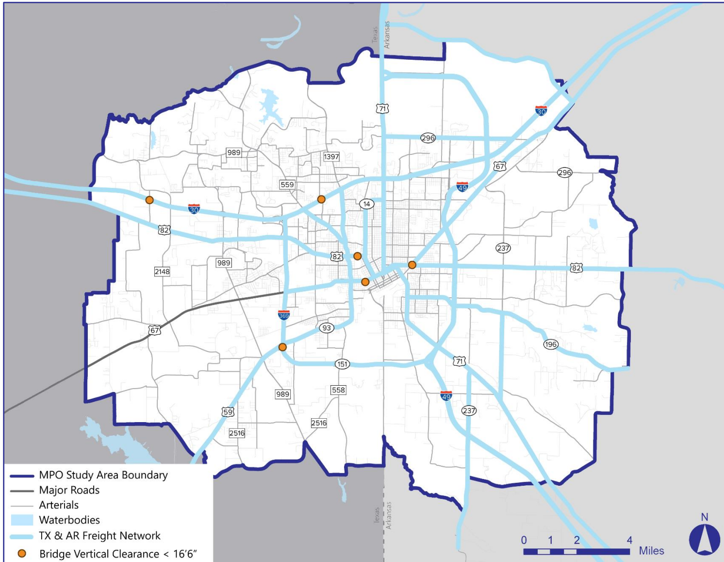
Figure 11: Bridge Vertical Clearance; 2019; from TxDOT
