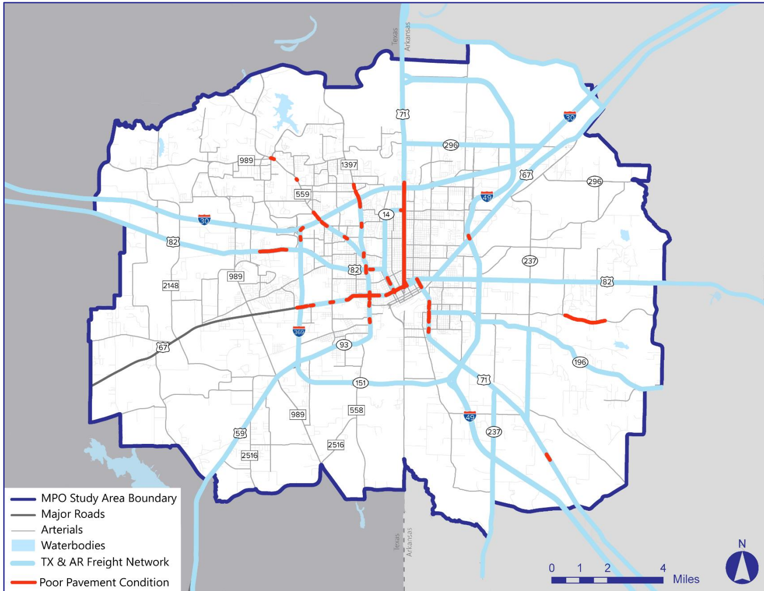
Figure 12: Poor Pavement Condition; 2017; FHWA Highway Performance Monitoring System
